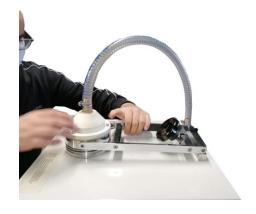
Mask testing kit is exclusively designed in compliance with the Standard EN14683:2019 and ASTM F2100:2019, but it keeps the standard test method for the determination of the air permeability on fabrics in compliance with UNI EN ISO 9237, ASTM D-737, etc.
