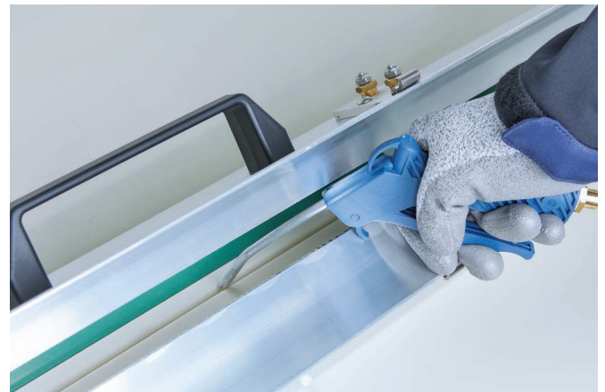
Backside cleaning with air pressure
