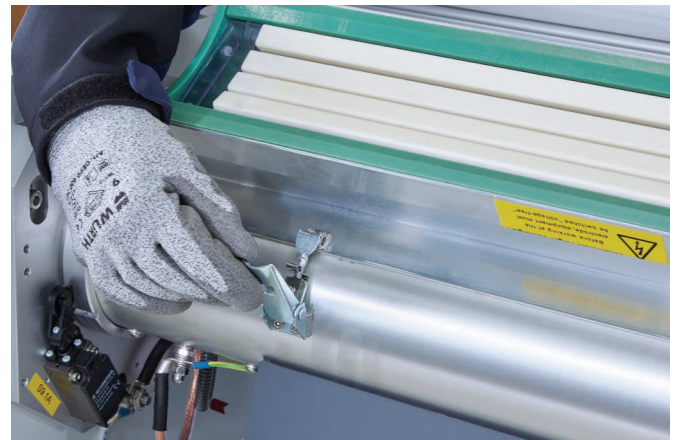
Simple and safe operation – Easy fixation with snap locks
