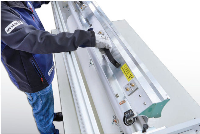
Tool-less removal of the electrode system
