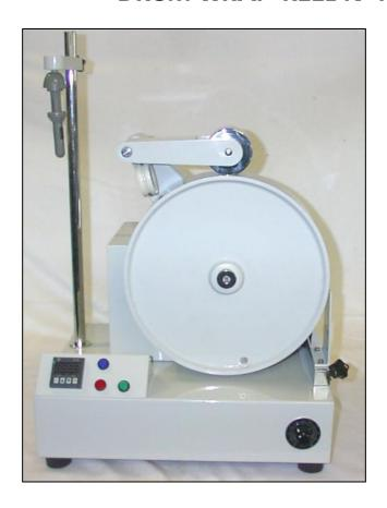
This equipment is specially designed to determine the count of slivers and roving during the process preparation. It is provided with an oscillating cylinder adherent to the drum, a. counter, a cutting device to obtain an accurate measure, a speed adjusting device and a bracket to hold bobbin.
